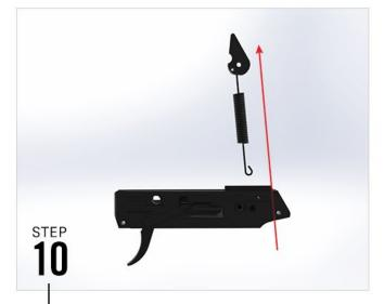
Remove hammer and spring assembly.
