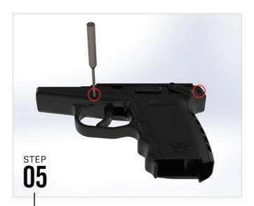
Using a 3/32" punch, remove the frame pins.
